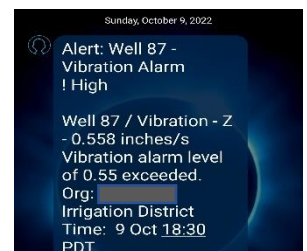
Example SMS text alarm pushed to phone
